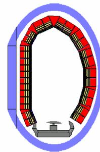
Fig.6. Elevation of HCSB-DEMO MCNP model
