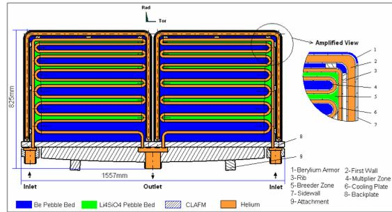
Fig.4. Cross-section of HC-SB DEMO Blanket
